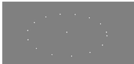
*The 3D edge points from a circular object. Can be located by PlaneFit3D*
